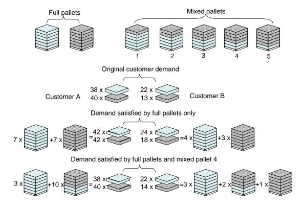
Figure 1: Example for the use of mixed pallets
