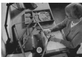
FIGURE 3 Tracing the working drawing on the table of a pantograph; while tracing the outline of the drawing, the design was cut at a reduced size into a wax coated glass plate. Reproduced with permission of Monotype Imaging.
